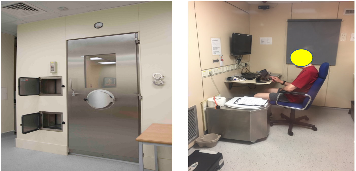
Figure 4.1 Outside (left) and inside (right) of one of the respiration chambers used in this study.
