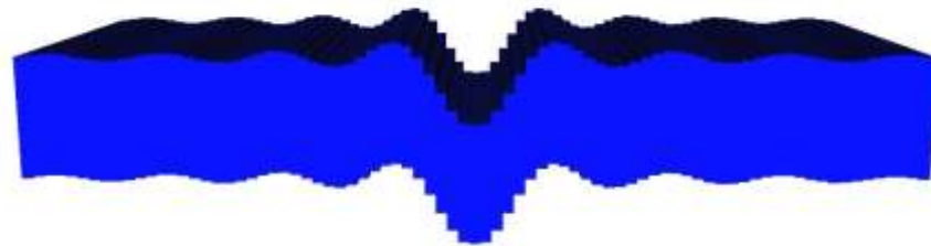
Figure 3.11. Aquifer model used for numerical simulation and analytical calculation. All figures are exaggerated by a factor of 25 in the z-direction.
