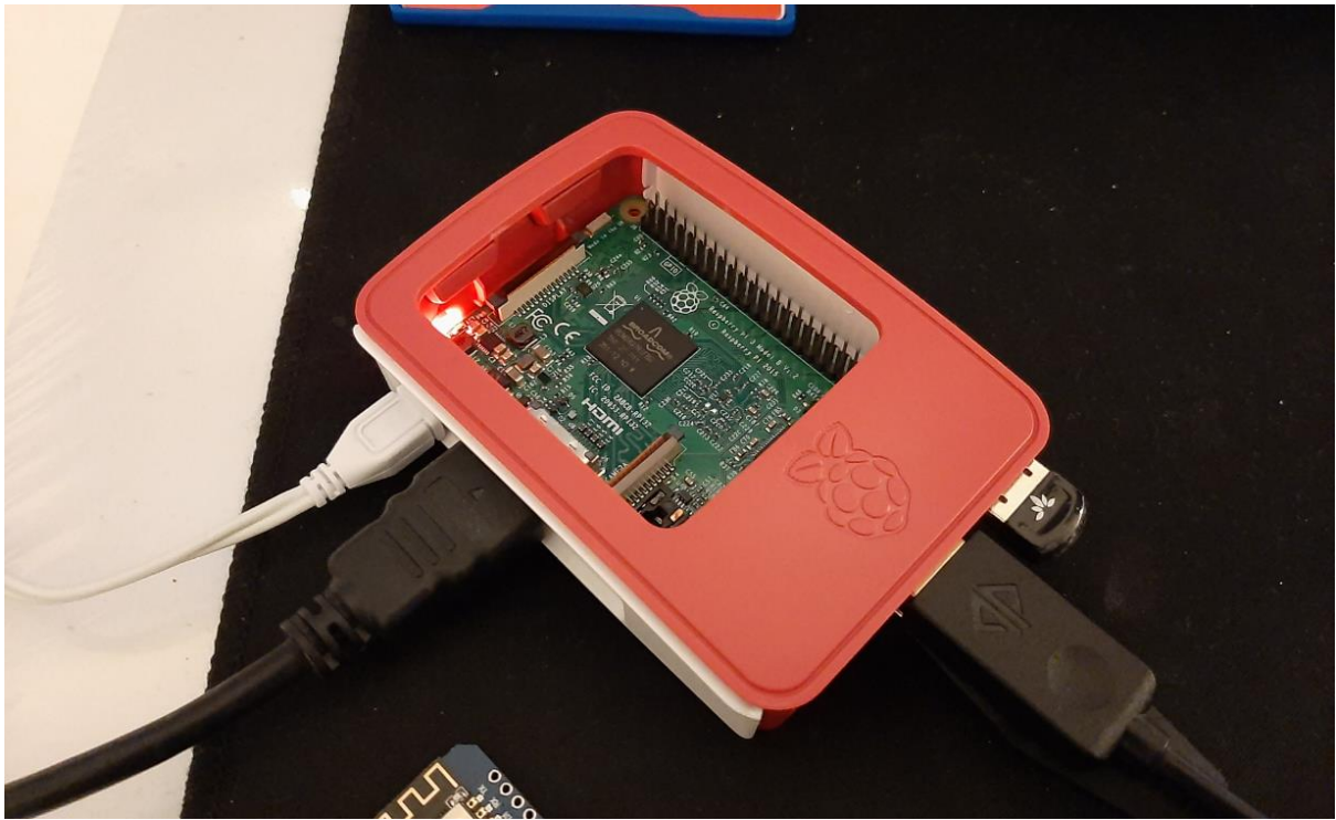
Figure 65. The low-powered raspberry pi3 used in the experiments
