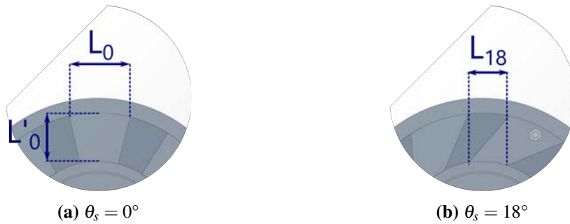
Figure 4.8 Characteristic lengths extracted from the swirl generator for \theta_s = 0^\circ (a) and \theta_s = 18^\circ (b). The dimensions indicated are used in Table 4.1.
