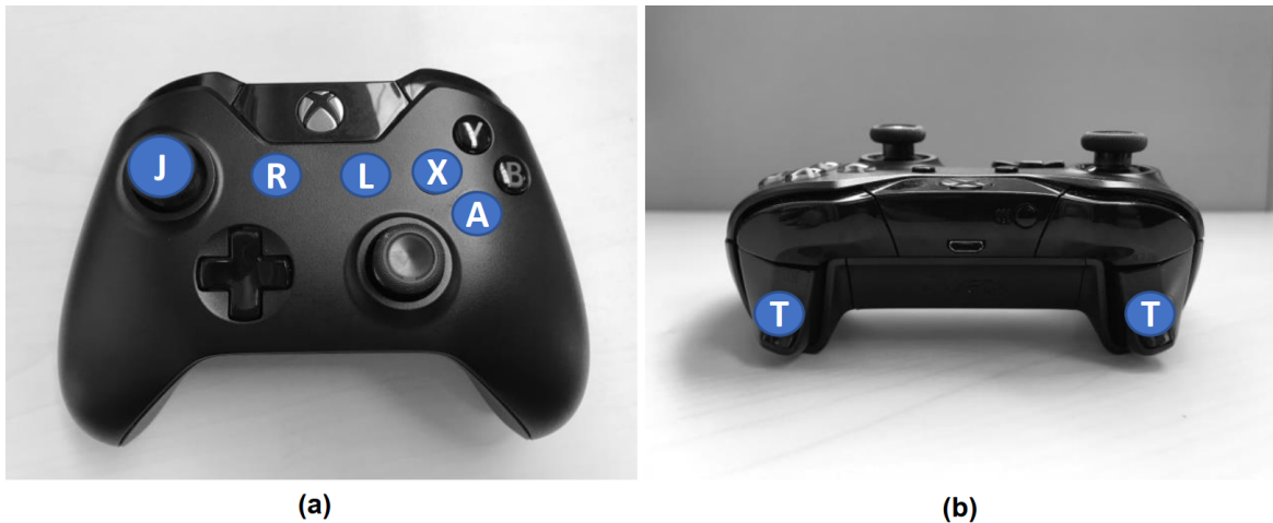
Fig. 3.7 The Xbox controller: (a) shows the top view with the left-hand joystick [ J ] used to control the 2D movement on the X-Z plane whereas (b) shows the front view with the two triggers [ T ] responsible for vertical movement along the Y axis. The other action buttons indicated in (a) have the following meanings: [ R ] for reload of the visualisation; [ L ] for loading next dataset; [ A ] for selection of an interactive item; and [ X ] for moving or rotating the scatter plots.
