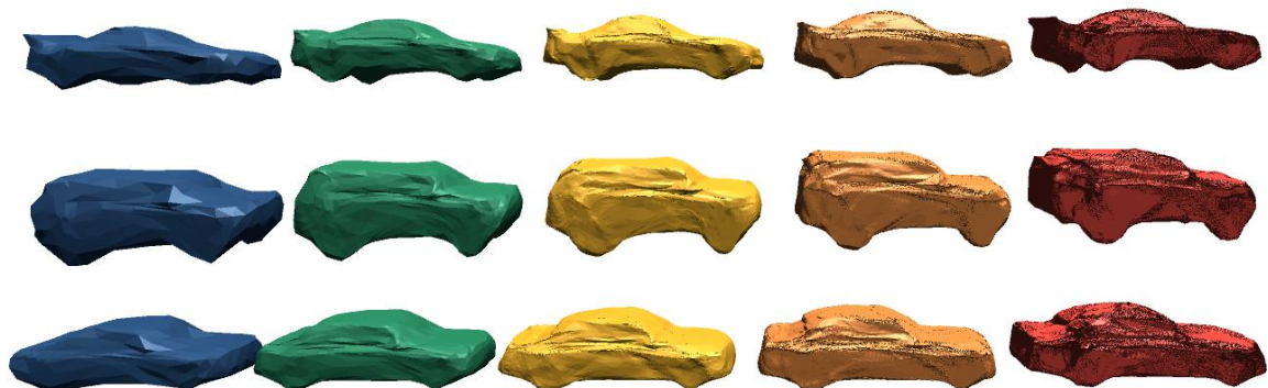
Fig. 1.7 A range of 3D meshes of cars generated with the Hypernetwork method [145] as they are seen by the headset wearer in the VR environment [157]. The number of triangles in the meshes, i.e. their quality, grows from left to right.
