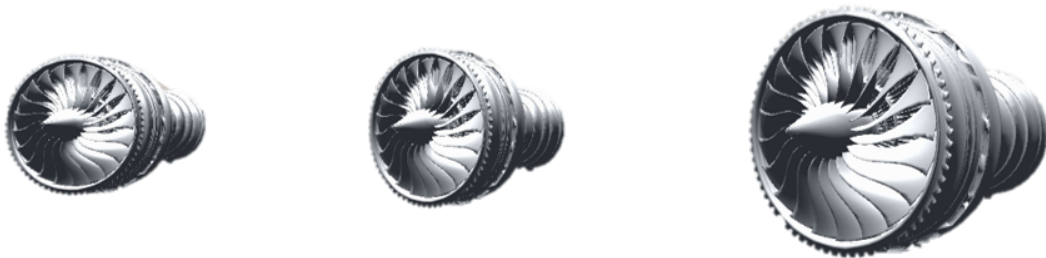
Fig. 1.5 An array of 3D CAD models [57] of aeroengines used as a basis for a VR-based digital twinning application in aeronautics [154]. The figure was generated within the AeroVR environment [157].
