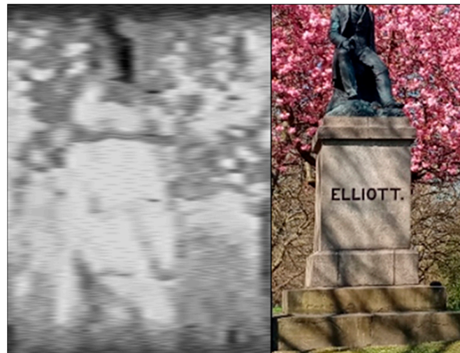
Figure 12. Spatial dataset captured of a statue over a longer working distance (ca. 20 m). Whilst this dataset is of poorer quality than others captured with this instrument, the target object can be identified highlighting the potential for the capture of landscape-style scenes in the future.
