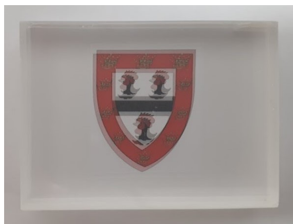
Figure 2.10: Image of a calcite crystal, used for Neutron Reflectometry, on top of a piece of paper displaying the crest of Jesus College, Cambridge. The anisotropy of the crystal structure leads to two refractions of light, producing two images, referred to as birefringence.
