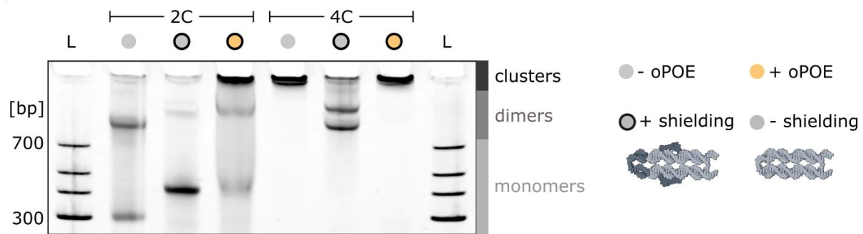
Figure 7.3 PAGE analysis showing the effects of additional ssDNA overhangs (“+/- shielding”) as well as addition of a 0.5% octylpolyoxyethylene surfactant (“+/- oPOE”) on the aggregating behaviour of cholesterol-modified 4H structures.
