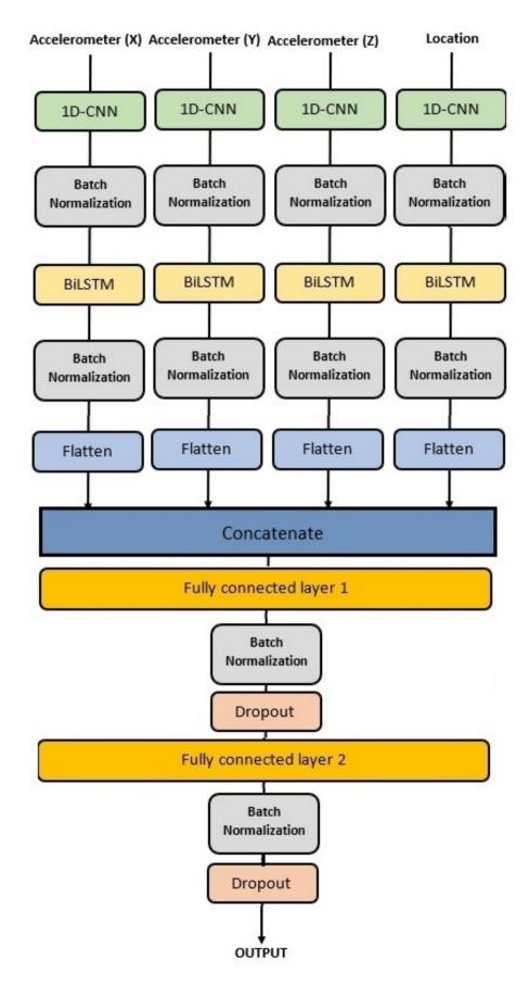
Figure 6.1: The overall architecture of the 1DCNN-BiLSTM smoking events prediction model.
