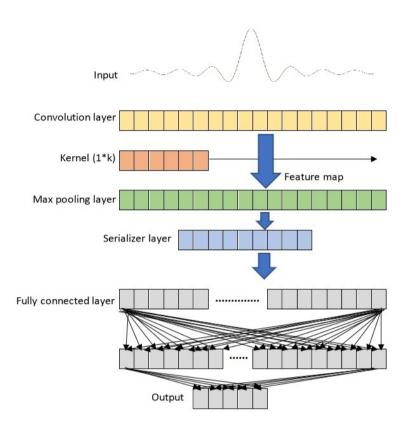
Figure 3.5: General 1D-CNN design based on Kim et al. (2020)
