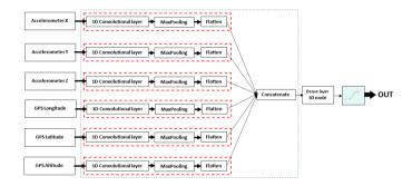
Figure 9. One-dimensional convolutional neural network (1D-CNN) model architecture.
