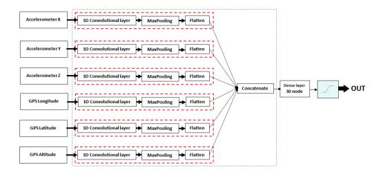
Figure 5.1: One-dimensional convolutional neural network (1D-CNN) model architecture (Abo-Tabik et al., 2020)
