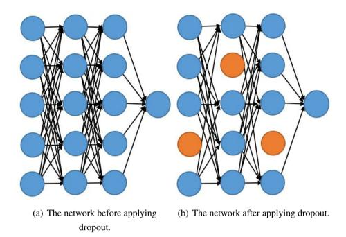
Figure 3.4: Applying the dropout method on DNN.
