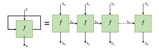
Figure 3.6: Basic architecture of RNN based on Zhao et al. (2017)
