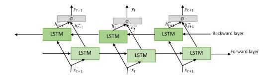
Figure 3.8: Illustration of BiLSTM network based on Zhao et al. (2017)
