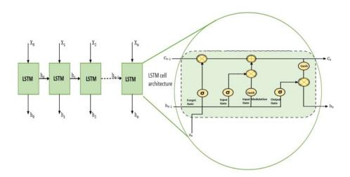
Figure 3.7: LSTM cell architecture based on Zhao et al. (2017)
