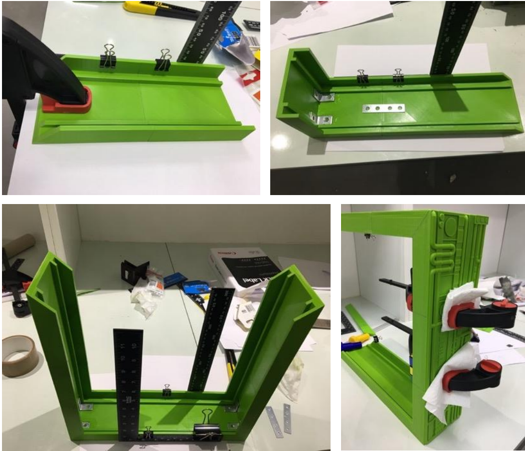
Fig. 31. 3D printed frame being assembled
