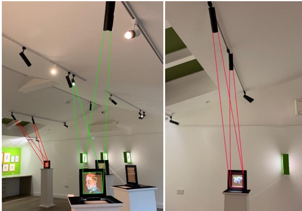
Fig. 21. Two views of the studio setup. The green lines indicate the geometry of luminaires placed on opposite sides of the hologram. The red lines mark the lights placed on the same side of the hologram.
