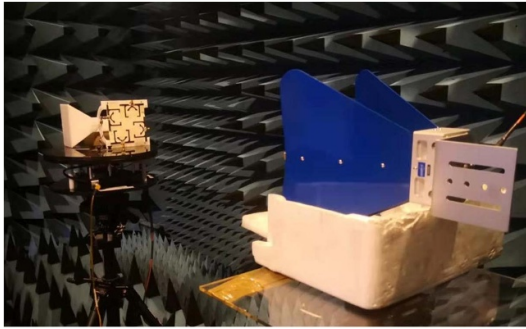
Figure 6. Antenna measurement set up with a horn antenna in anechoic chamber, the distance between the horn antenna and the MIMO antenna under test is 0.8 m.
