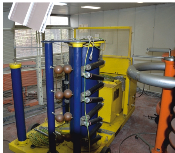
Figure 5. Marx generator set to pulse voltage 0.2/10 \mu s
