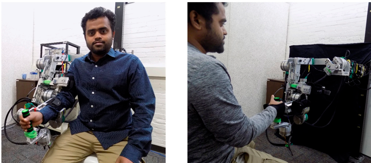
Figure 17. On the left , the subject is wearing u-Rob as an exoskeleton-type setup for joint-based exercises, whereas on the right , the subject is wearing u-Rob as an end-effector-type setup for end-point exercises.
