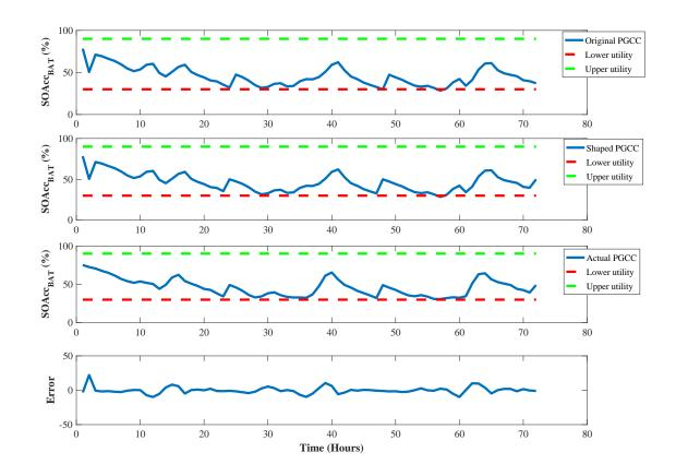
Fig. 4.11 PGCC shaping and BAT response for 72h under non-Gaussian uncertainty
