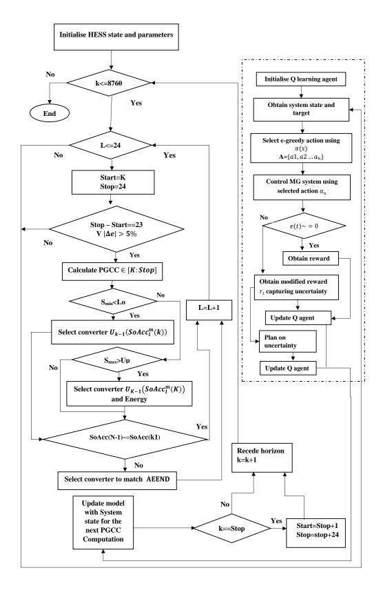
Fig. 6.2 RL+Adaptive Power Pinch Algorithm
