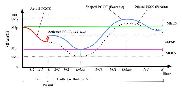
Fig. 3.2 Shaped PGCC with respect to Lower Pinch
