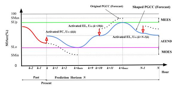
Fig. 3.5 Completely Shaped PGCC in the Predictive Horizon
