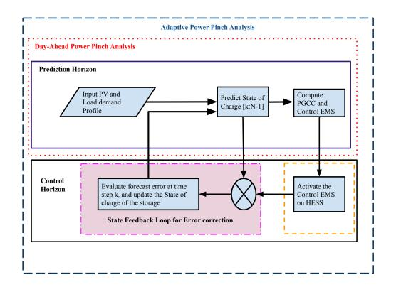
Fig. 1.3 Schematics of the Adaptive Power Pinch Analysis EMS for HESS [46]
