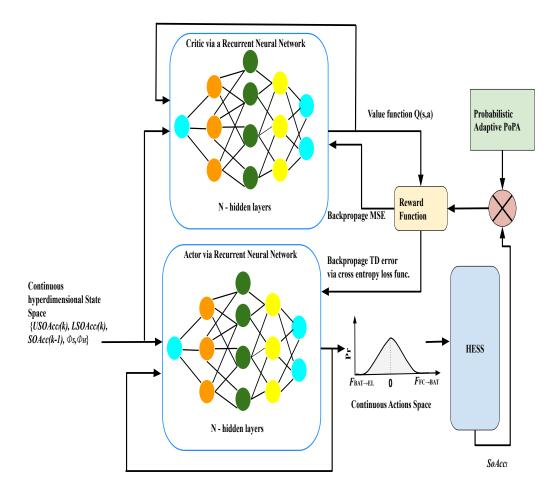
Fig. 6.4 Actor-Critic Probabilistic Adaptive PoPA Schematic
