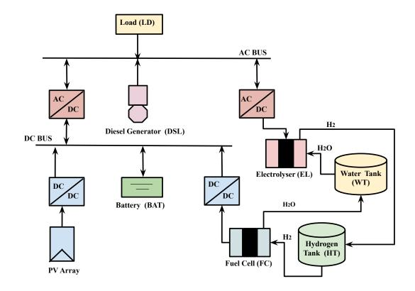
Fig. 1.2 Schematics of the Islanded HESS [17] used as a case study
