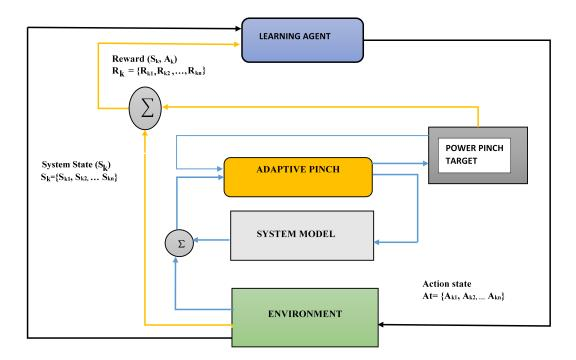
Fig. 6.1 Reinforcement Learning Adaptive Power Pinch Schematic
