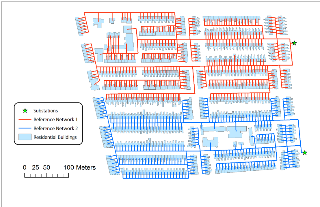
Figure 6.34. Generated electricity network in test area 2, based on ITN road network (Contains OS data © 2018).
