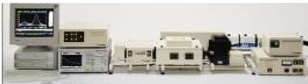
Figure 9: Laser set up used to measure transient absorption spectra.
