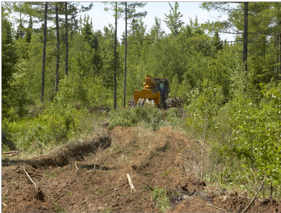
Skidder Soil Disturbance (Photo by Pamela Wells)
