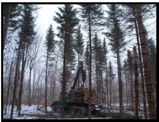
Precommercial thinning stand with cut-to-length harvest system (left); no precommercial thinning stand with whole tree harvest system (right). Photos courtesy Patrick Hiesl and Brian Roth.
