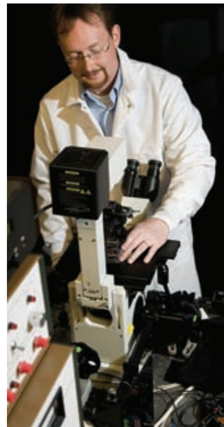
The FPALM microscopy system breaks a fundamental limit on the resolution of lens-based microscopes, known as the diffraction barrier, which has existed for more than 100 years.
