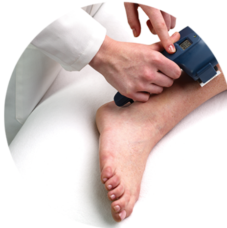
Figure 7. DPNCheck by NeuroMetrix is a device targeted at measuring sural nerve conductance. Reproduced from Ref [19].
