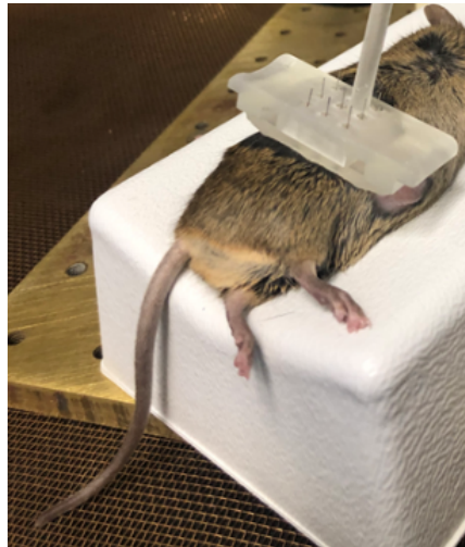
Figure 17. Image of the mouse and needle array positioning that was used in the experiment to test design dimensions and recording from a needle array. Array designed and printed by Julia Towne.
