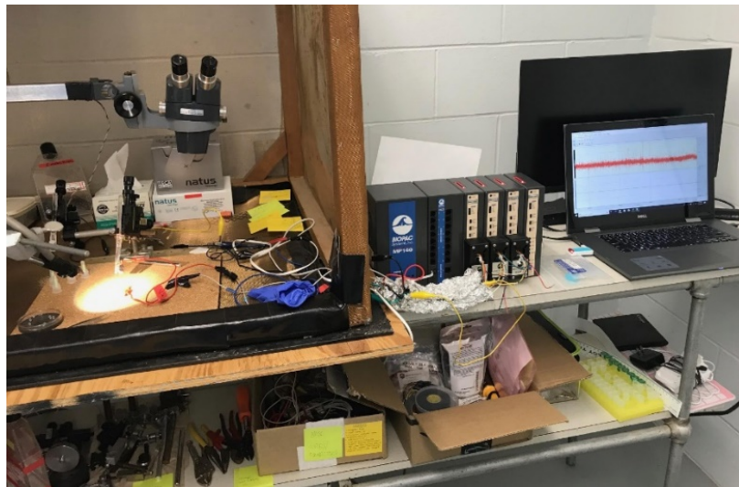
Figure 11. Recording setup with the Faraday cage, BIOPAC hardware, and the laptop with the necessary software. Reproduced from Brooke Villinski.
