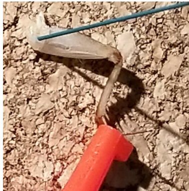
Figure 24. Experimental setup for the cricket leg test with the Natus commercial electrodes pictured. The nerves were stimulated mechanically, with the recording electrode in the Coxa and the ground in the Tarsus. Reproduced from Brooke Villinski.
