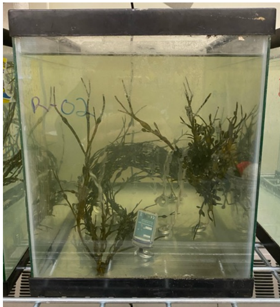
Figure 3. Photograph of rockweed treatment tank filled with Instant Ocean solution and containing a HOBO logger and a weighted down rockweed individual.
