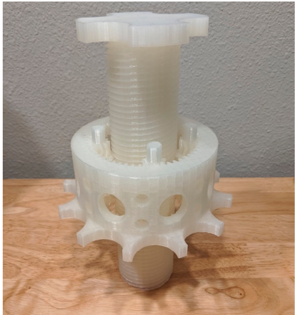
Figure 1. Fully 3D-printed and assembled roller screw assembly. Printed on an open source Prusa Mk3S in natural PLA at 0.2 mm layer height.
