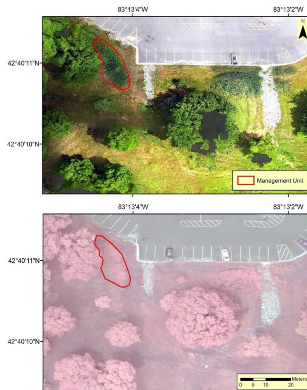
Figure 4. Overview imagery of management site 129. DJI Phantom 3 optical RGB (top) and MAPIR near infrared false color composite (bottom) orthophotos.
