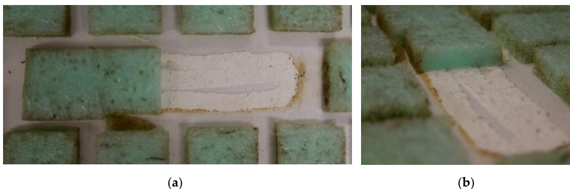
Figure 1. Cut away view showing adhesive underneath foam attached to c-Si-based flexible photovoltaic (PV) module: (a) top view and (b) orthogonal view.
