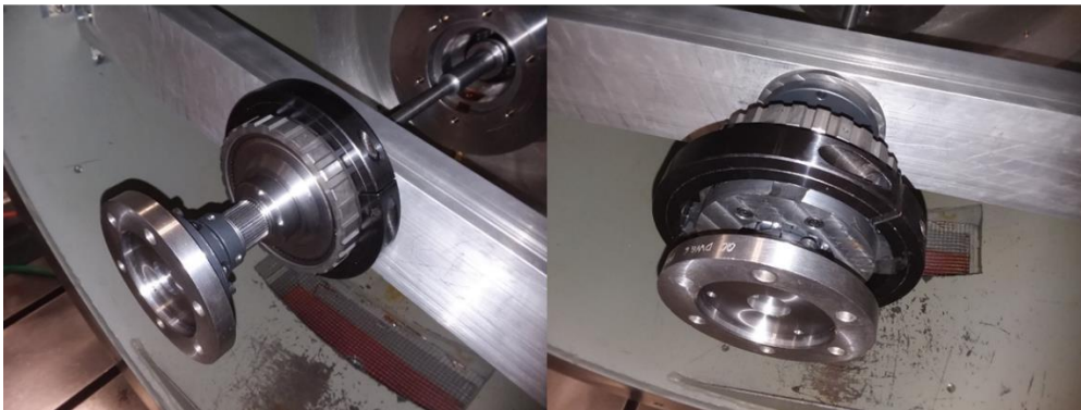
Figure 2.4. Sketches of the ring pTVA and the sun pTVA (top). Completed fabrication of ring pTVA (bottom left), and sun pTVA (bottom right). The absorber inertia in each configuration is the black shaft collar, which clamps around the rubber and the free spinning gear. The grounded gear bolts to a beam which runs across the diameter of the fixture.
