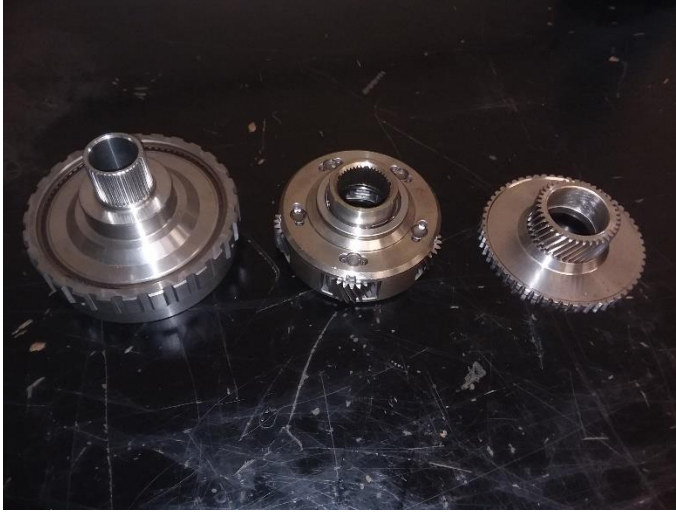
Figure 2.3. Disassembled planetary gear set from second generation Chevrolet Volt drive unit with 81 tooth ring gear (R) and 39 tooth sun gear (S).
