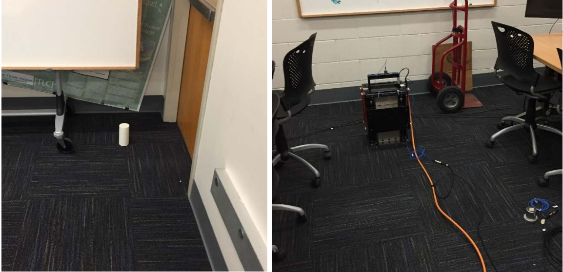
(a) The Origin in The Tested Floor (b) Shaker at Location L4
