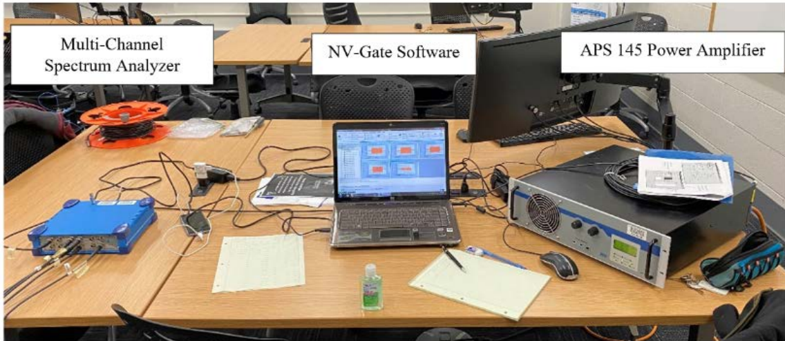
Figure 3.4: Multi-Channel Spectrum Analyzer, NV-Gate Software program, and APS 145 Power Amplifier
