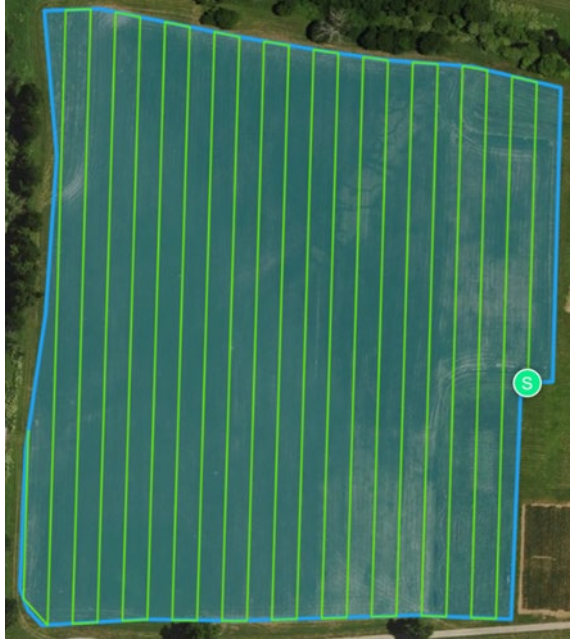
Figure 3.3 The image depicts field 1. The area highlighted in blue is the alfalfa field, and the green lines represent the path of the UAV.
