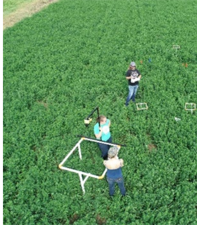
Figure 2.5 This image depicts how the 3D scans of the canopy at each quadrat were collected. The LiDAR sensor was attached to a frame and mounted onto the quadrat to acquire each scan.
