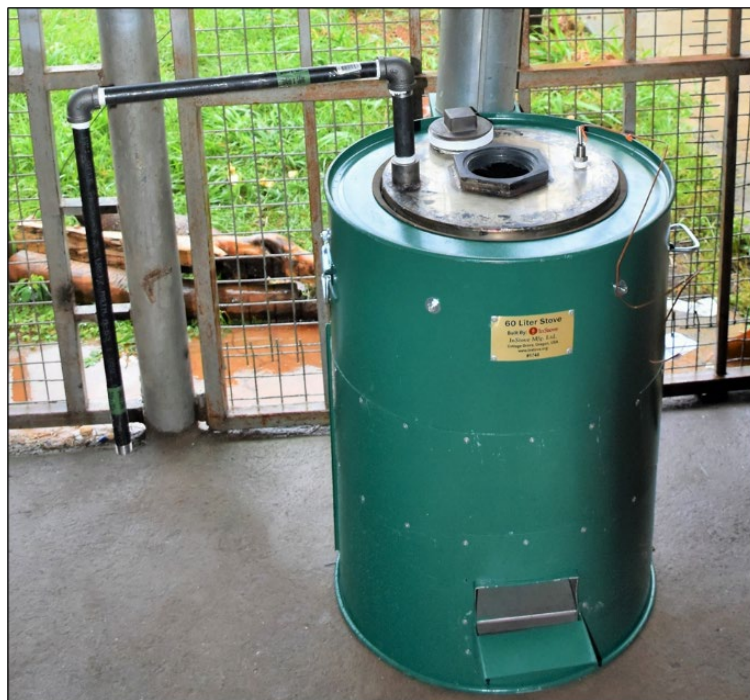
Figure 4.2. Photograph of the UKATS process for converting post-consumer waste plastic into fuel oil
