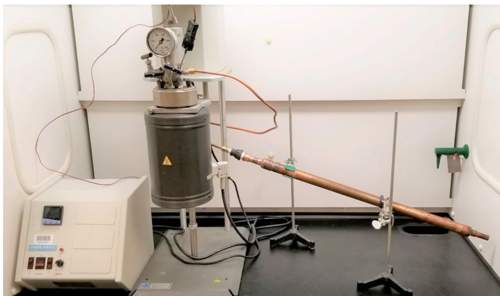
Figure 8.1. Parr reactor and Parr 4843 controller setup for slow pyrolysis experiments
