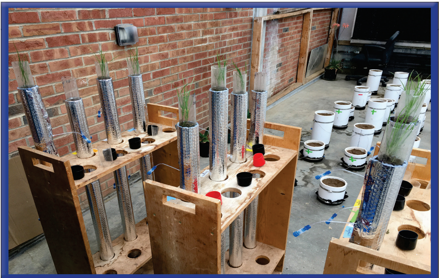
Soil cores were collected from a site in Princeton, KY, and after being fertilized, were seeded with annual ryegrass. All cores were wrapped in Reflectix insulated bubble wrap to prevent unrealistic soil warming and algae growth. (Photo Credit: Dr. Christopher Matocha)
