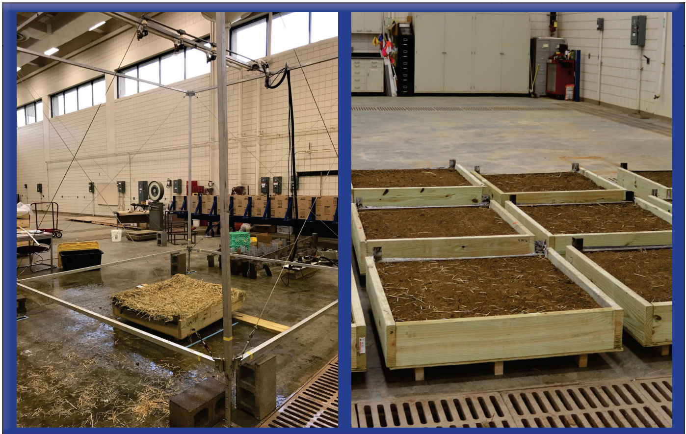
(L) Preliminary test of the rainfall simulator on soil box with straw cover. (Photo Credit: Dr. Brad Lee)
