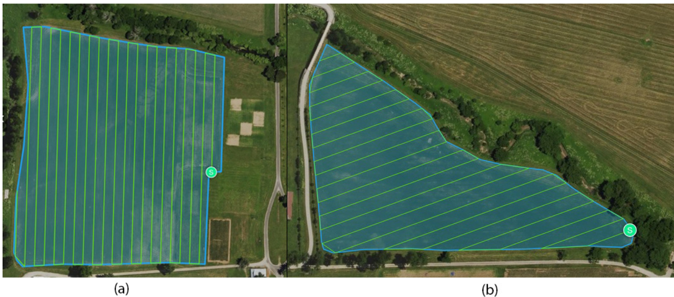
Figure 2. Field 1 (a) and Field 2 (b) outlined in blue. The green lines show the UAV path when following a mission to cover the entire field. The “S” indicates the starting point of the mission.
