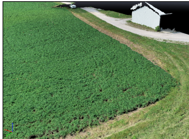
Figure 4. An isometric top view of a portion of a fully processed alfalfa model of field 1 flown on 4 June 2019 using 30–90° flight parameters. Only part of the nearby barn is modeled as the flights only recorded one side of the building.
