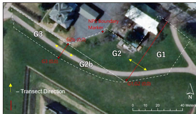
Figure 3. Map showing layout of survey grids and direction of data acquisition.
