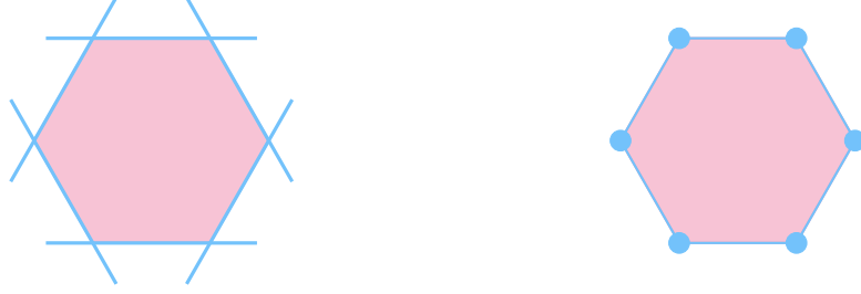
Figure 2.1: A hexagon as a bounded intersection of 6 half-spaces (left) and a hexagon as the convex hull of 6 vertices (right).
