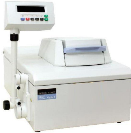
Figure 2.4: Pyris I DSC to measure the stress-free phase TTs [125].
