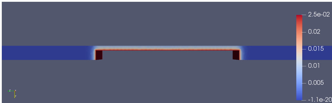
Figure 3.7: Electric potential from the solution of the Linearized Poisson-Boltzmann equation. The model uses both planes of symmetry, so only one quarter of the pore and reservoirs are shown. The electric potential boundary conditions are 25 mV at the membrane surfaces.
