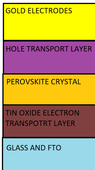
Figure 7: The layers of the fabricated device. The bottom layer, deposited first, is the electron transport layer comprised of Tin (IV) Oxide nanoparticles, Perovskite crystal of \text{Cs}_{0.05}(\text{MA}_{0.17}\text{FA}_{0.83})_{0.95}\text{Pb}(\text{I}_{0.83}\text{Br}_{0.17})_3 , Organic Hole transport layer, top electrode of gold. Figure 7 1: The layers of the fabricated device. The bottom layer, deposited first, is the electron transport layer comprised of Tin (IV) Oxide nanoparticles, Perovskite crystal of \text{Cs}_{0.05}(\text{MA}_{0.17}\text{FA}_{0.83})_{0.95}\text{Pb}(\text{I}_{0.83}\text{Br}_{0.17})_3 , Organic Hole transport layer, top electrode of gold.
