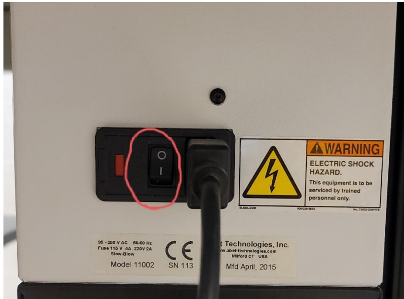
Figure 19 1: Back Power switch of Solar Simulator.
