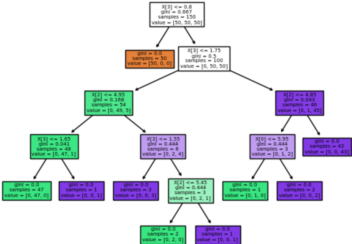
Figure 2: An example of a decision tree. Decision trees work by making binary decisions across a decision boundary. Each leaf node represents a classification label and the binary decisions that selected that label.
