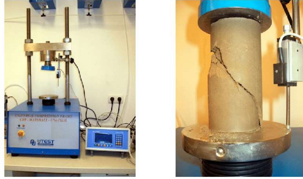
Figure 4. The unconfined compressive strength test
