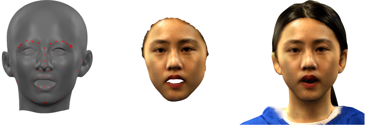
Figure 4.10: Face re-targeting result. The two left images show the input deformed face model and the re-targeted face part of the pre-scan, respectively. The face vertices of the body model are replaced by their deformed counterparts, as shown in the right image.
