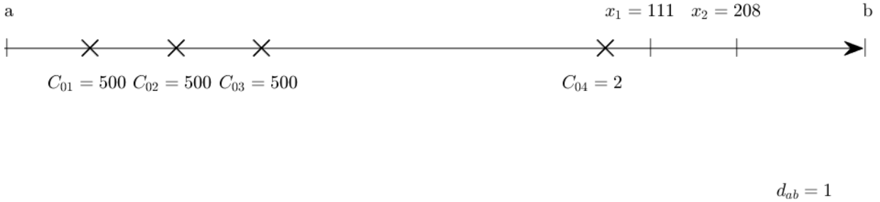
Figure 2.4 River reach flowing from a (left) to b (right) showing the location of four pollution sources (X) and two sampling points (+). The pollution sources consist of three large farms with 500 animals each on the upstream end, and a small farm with 2 animals on the downstream end. The IDW interpolation predictor calculated at two sampling points downstream of the small farm have values of x_1=111 and x_2=208 . These values increase moving downstream and away from the sources, which lacks physical meaningfulness.
