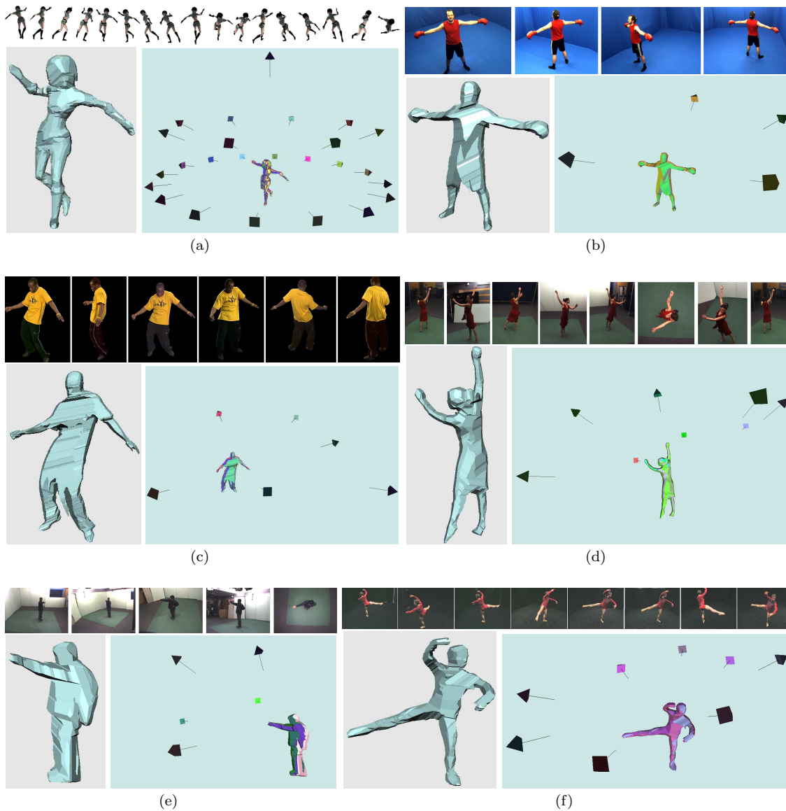
Fig. 13 Metric 3D reconstructions from six different datasets – (a) Kung-fu, (b) Boxer, (c) Dancer2, (d) Dancer1, (e) Man and (f) Ballet. The recovered camera network is visualized along with a visual hull reconstruction (computed using the approach of [10]) of the subject in each case.
