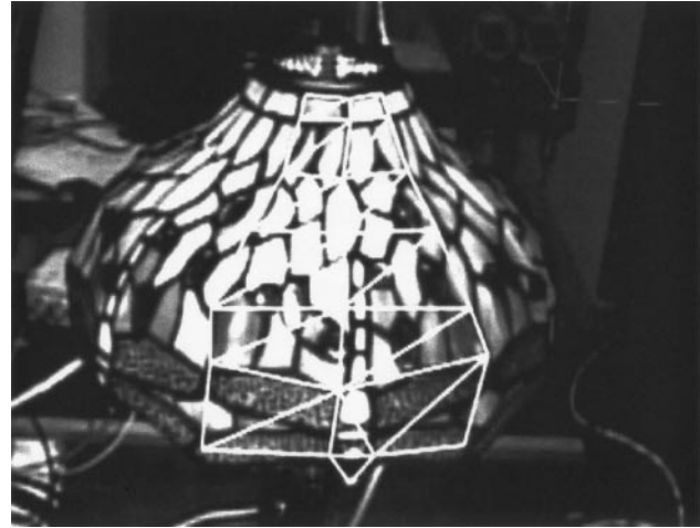
Figure 4. Wireframe model of a 60 deg. segment of the lamp overlaid on the video image of the lamp.
