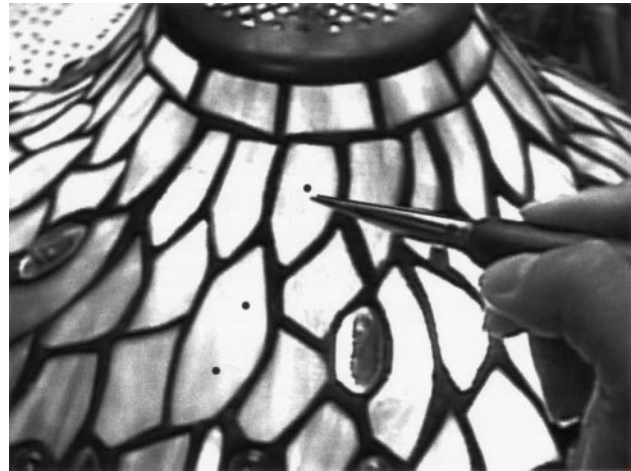
Figure 2. Sampling the geometry of a Tiffany lamp shade with the probe. The dark dots represent the acquired points. A dark line segment is rendered over the tip of the acquisition probe.
