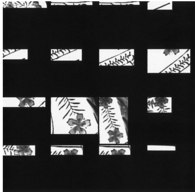
Figure 8. Stored texture array. These are some of the textures that are used to render the teapot model interactively. Each rectangular texture corresponds to the bounding box of a triangle.
