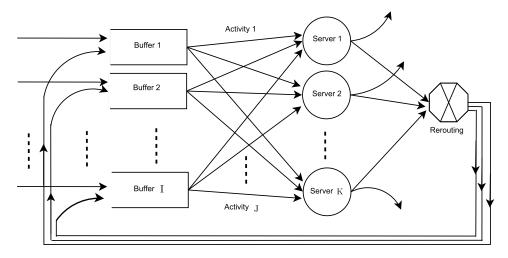
FIG. 1. A network with I buffers, J activities, K servers and probabilistic routing (given by the matrix P).
