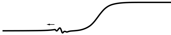
FIGURE 1.2. In the frame moving with the front, a small, sufficiently localized perturbation is transported to -\infty .
