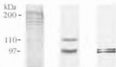
FIG. 1. Analysis of purified IF-2 chl by SDS-PAGE. Each sample contained ~50–60 ng of protein and 0.1–0.2 unit of TSKgel SF-5PW HPLC-purified IF-2 chl . First lane, IF-2 chl α1; second lane, IF-2 chl α2; third lane, IF-2 chl β. Samples were resolved on 6% polyacrylamide gels that were stained with silver as described (18).
