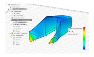
**Figure 24.** Modal Frequency test at 28.15 Hz
