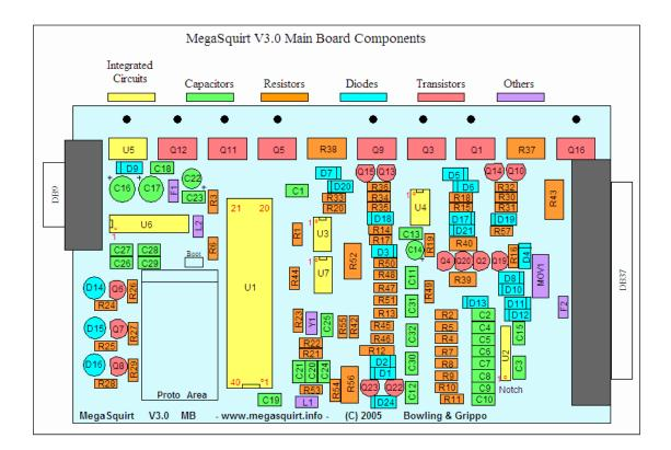
Figure 13. Main Board Components for MegaSquirt II version 3.0
