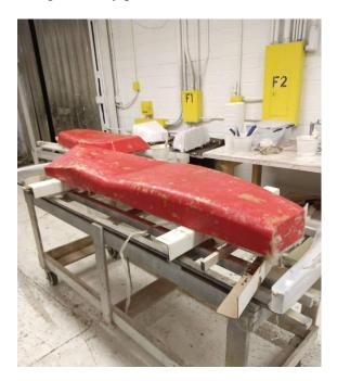
**Figure 5.** Right side body panel mold with initial fiberglass layer
