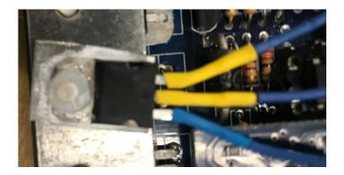
Figure 25. BIP373 Transistor modification for dual spark configuration
