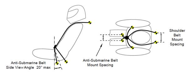
T.2.7.3 All Anti-Submarine Belts must be installed so that they go in a straight line from the Anti-Submarine Belt Mounting Point(s) without touching any hole in the seat or any other intermediate structure until they reach:
