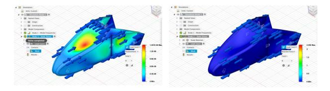
Figure 20. Static Stress test on Displacement
