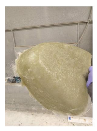
Figure 7. Nose panel after being detached from the mold
