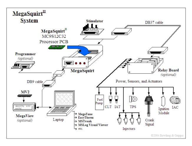
Figure 27. MegaSquirt System Overview with MS2 processor [1]
