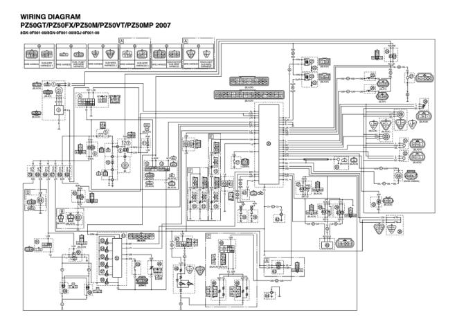
Figure 29. 2007 Phazer Wiring diagram with all relay and fuse systems
