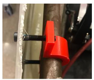
Figure 10. 3-D body panel mounts
