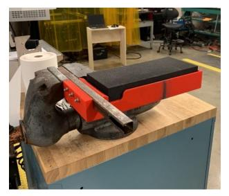
**Figure 16.** The 3-D printed headrest is composed of three parts with the interface being secured using aircraft grade epoxy
