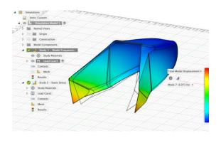
**Figure 22.** Modal Frequency test at 8.973 Hz
