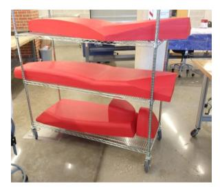
Figure 3. First stages of CNC machining the foam mold pieces that will be glued together
