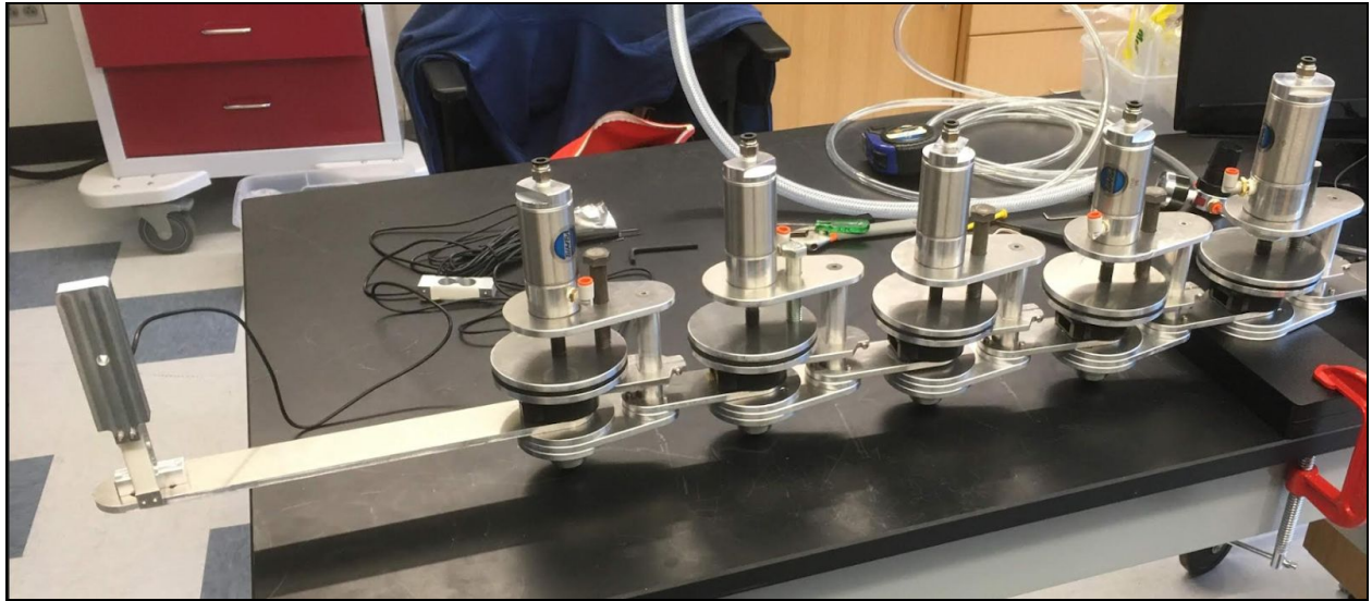
Figure 3. Physical prototype machined and assembled by Ryan Hodge. Note that only five joints are shown in the figure because of limited time for the project and availability of the staff to help during remote learning. This does not affect our testing for the force and torque requirement, which is described in section 3.2.2.
