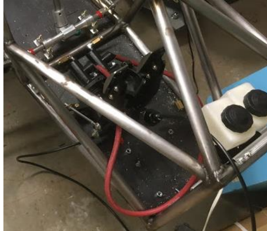
Figure 7.1.6: Brake pedal assembly complete with master cylinders and remote brake fluid reservoirs
