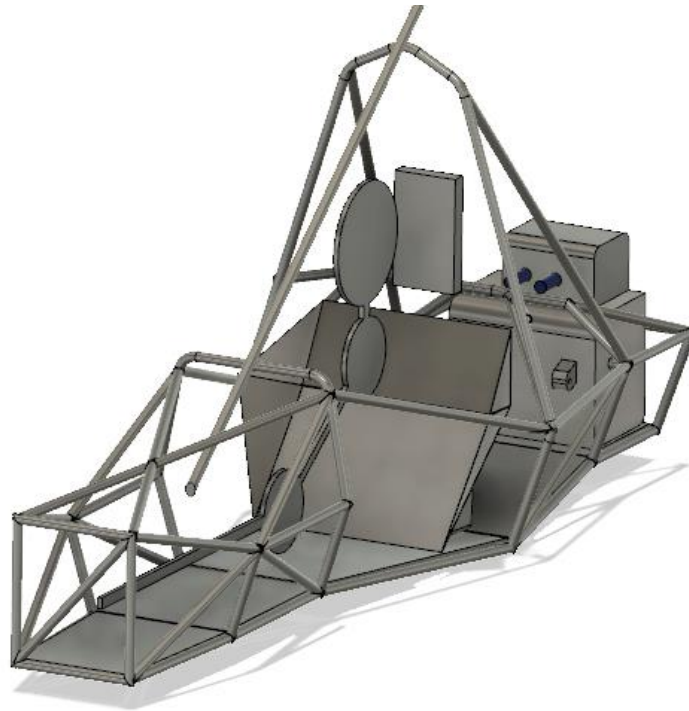
Figure 2.1.8 Isometric view of the PERCY model fit to the seat pan
