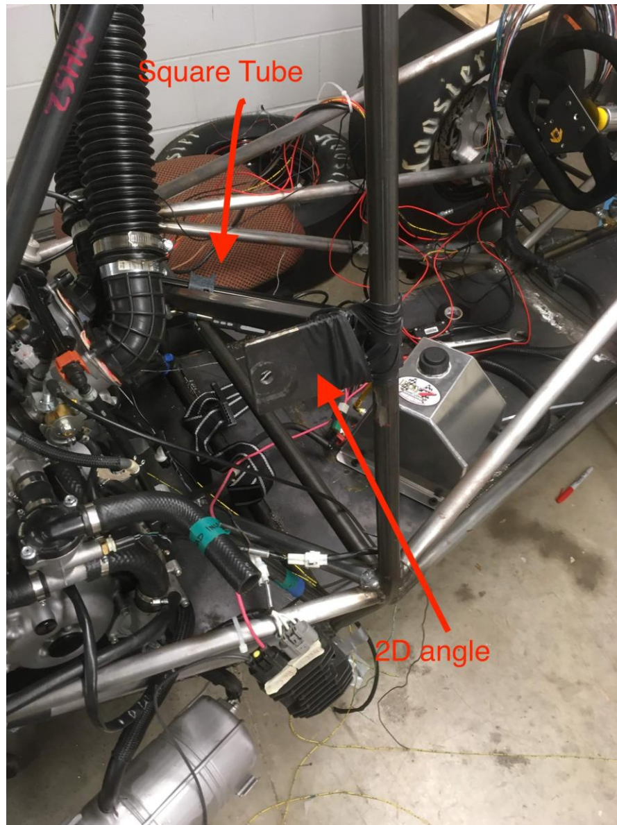
Figure 7.1.3: Square tubing and position
