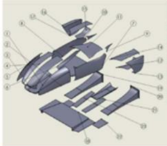
Figure 7.1.12: Individual parts of body panel design
