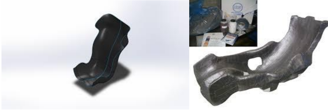
Figure 2.1.3 Carbon fiber seat (left) and creafom seat insert (right).
