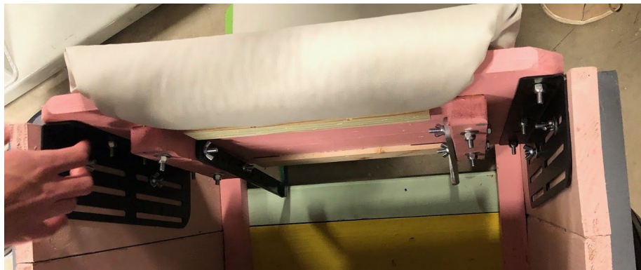
Figure 10. Chair bottom picture showing the metal supports attached to the wooden posts
