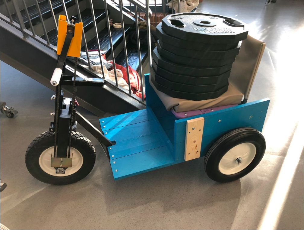
Figure 29: Prototype cart static load test with 360 lbs of weight on the seat
