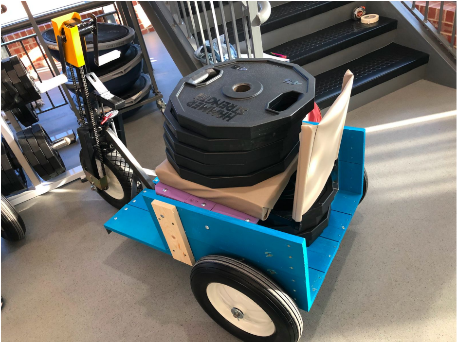
Figure 30: Prototype cart static load test with 225 lbs of weight on the seat and 100 lb of weight in the basket
