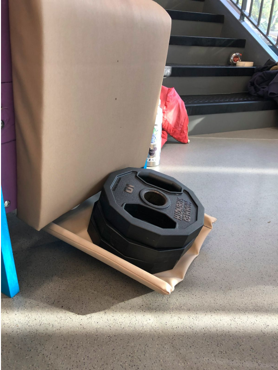
Figure 33: Prototype cart with 30 lbs of weight on the fabric
