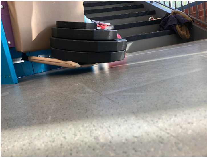
Figure 32: Prototype cart with 100 lbs of weight on the metal supports
