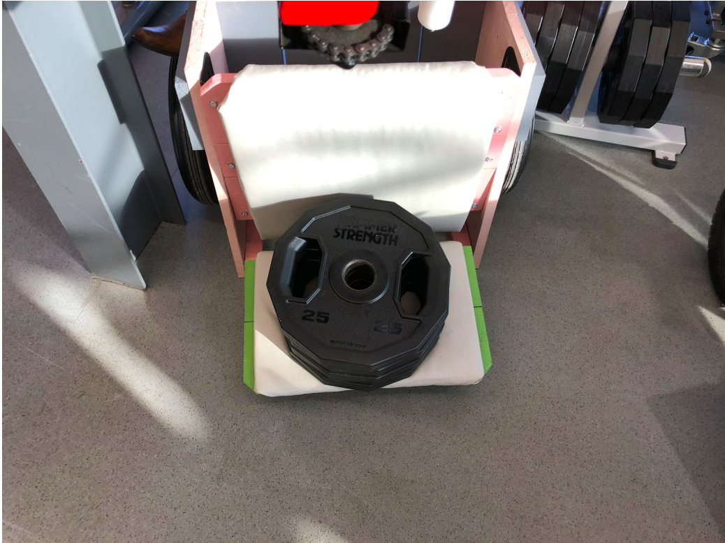
Figure 31: Reference cart with 100 lbs of weight on the chair back
