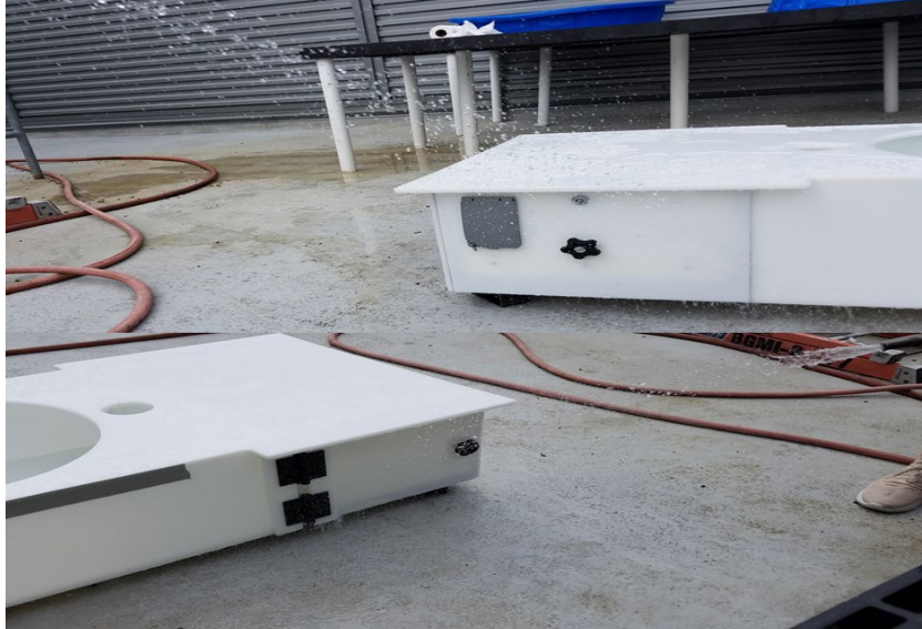
Figure 4: Top image is electronics compartment and USB cover, bottom is the electrolyte powder compartment, and load cell in within the base getting submerged.
