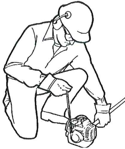
Figure 4: A picture from Shindaiwa T272 user manual showing recommended posture for using recoil cord-pull mechanism [4].
